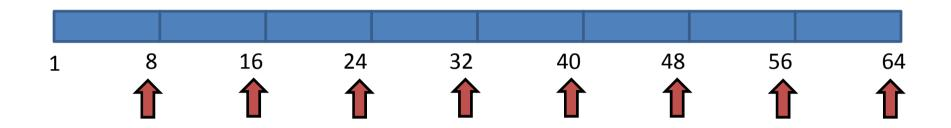
Parity bits, not used during DES encrypt / decrypt, hence 56 bit actual key
